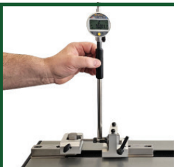
Setting 2-point bore gauges
